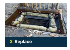
Once the LavaSorb™ boom basalt fibers are saturated, they can be wrung out with a wringer and the booms can be placed back in the pit with approximately 90% of the original capture volume. Otherwise, the booms can be disposed of according to local regulations.
