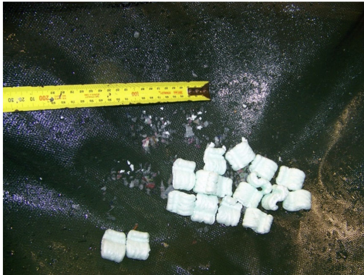
Figure 10: Escaped Solids – LittaTrap™ at 15 L/s
