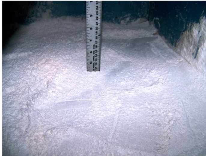
Figure 4: Sediment Pre-loading of Sump
