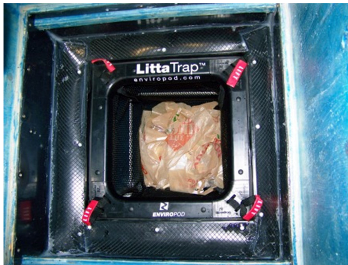
Figure 5: LittaTrap™ Scour Test Preload
