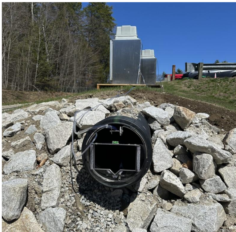
Figure 8. Outlet pipe fitted with a Thel-mar V-notch weir for effluent flow measurement; the two ISCO autosamplers stand on the pallet behind.
