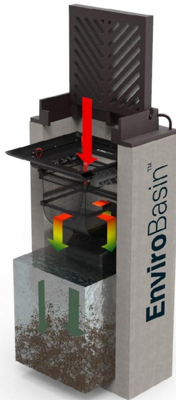
Figure 1. The EnviroBasin in operation: stormwater drops through the grate, the Energy Deflector reverses and spreads the flow across the sump, and sand and grit settle out while gross solids are held in the basket.
